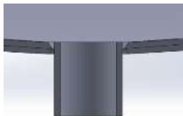
(C) Create groove at nozzle joint
