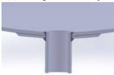
(E) Weld joint at nozzle to head dish
