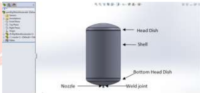
(B) 3D modeling of pressure vessel
