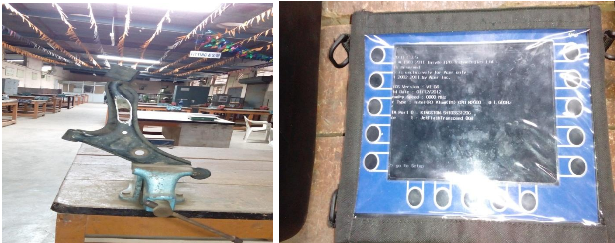
Fig: testing of control arm with FFT analyzer
