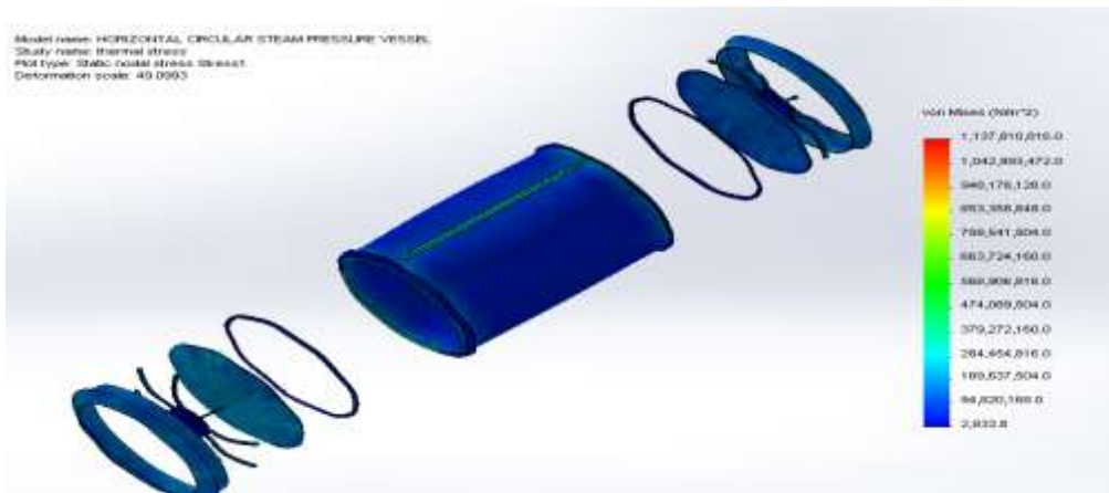
Fig 4.9 Von-Mises stress distribution on pressure vessel due to thermal loading in 5mm thk. shell.
