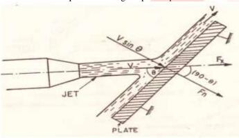
If the plate is smooth and if it is assumed that there is no loss of energy due to impact of the jet, then jet will move over the plate after striking with a velocity equal to intial velocity i.e., with a velocity V. Let us find the force exerted by the jet on the plate in the direction normal to the plate. Let this force is represented by F
