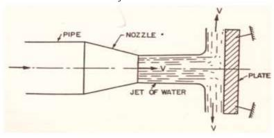
Force exerted by the on a stationary vertical plate Force exerted by the on a stationary vertical plate. The jet after striking the plate, will move along the plate. But the plate is at right angles to the jet. Hence the jet after striking will get deflected through
