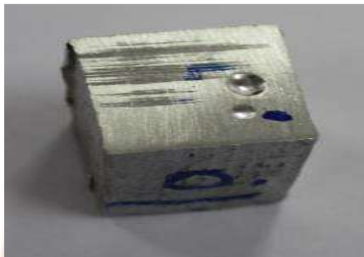
Figure 9: Hardness Test Specimens after test
