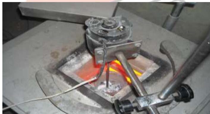
Figure 4: Stir casting setup
