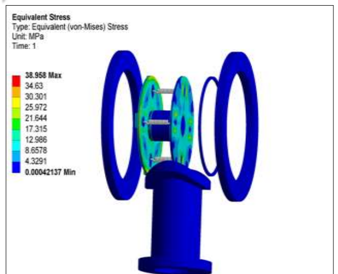
Figure 12 : Equivalent(von-Mises) stress for case 2
