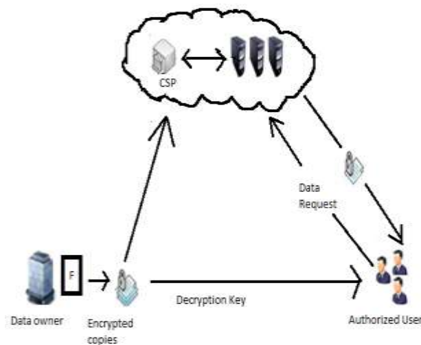
Fig. System Architecture
