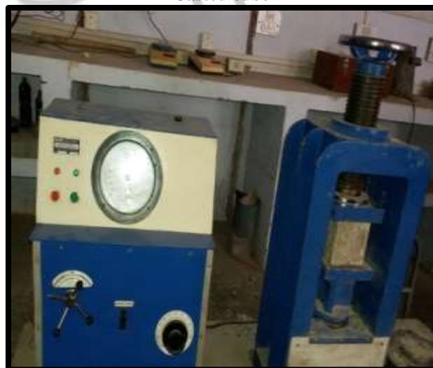
Geopolymer cubes being testing on compressive strength testing
