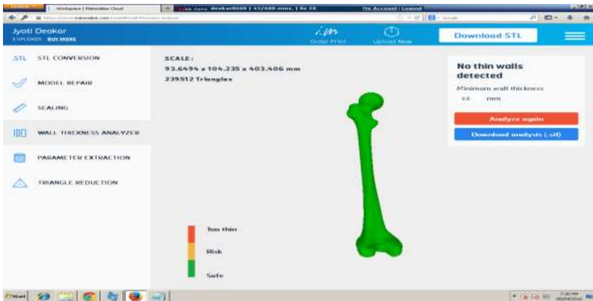
Fig. 6. Preparation of STL File for Prototyping
