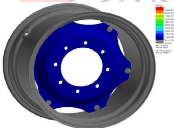
Figure 10: Optimized damage plots at the failure location
