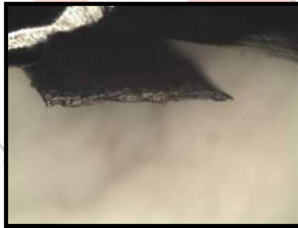
Fig-4 Cross-section of chip of Ti6Al4V at cutting speed of 300 RPM and feed rate of 0.25 mm/rev
