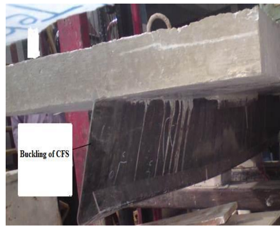
Figure (14): Typical large-scale test specimen (b6) failed due to buckling of CFS at support.
