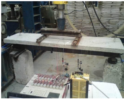
Figure (3): Large-scale test arrangement for composite beam.
