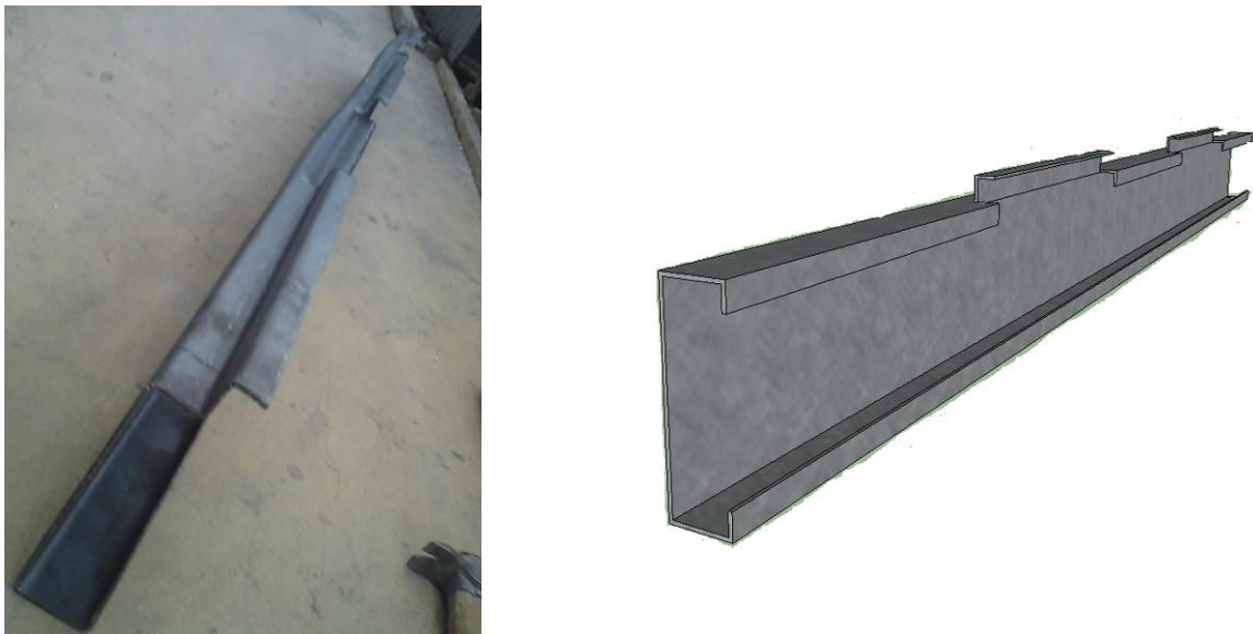
Figure (1b): Partial bent-up half flange of channel as shear dowel.
