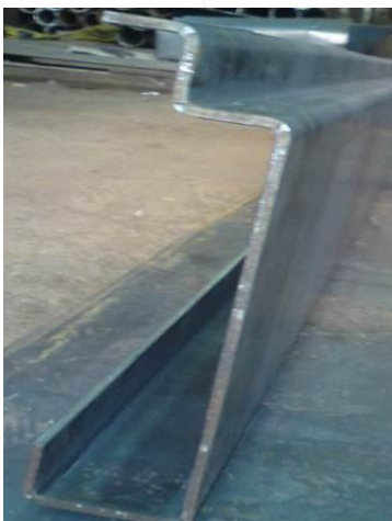
Figure (1a): Bent-up half flange of channel along beam as shear dowel.
