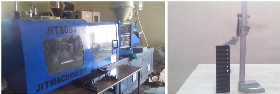
Fig 2 (A) J.I.T. Injection Molding Machine (B) Shrinkage measurement with help of vernier height gauge
