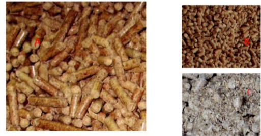
Figure 6. (A) Good quality pellets; (B) medium quality pellets; (C) poor quality pellets [3]
