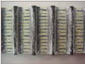
Figure 19. Extreme wear from abrasion[2]
