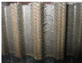
Figure 14. Extreme tooth wear from worn sprockets[2]
