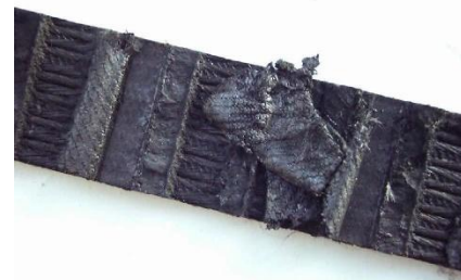
Figure 21 Melting from high temperature operation [1]
