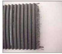
Figure 23. Crimp failure due to debris [2]
