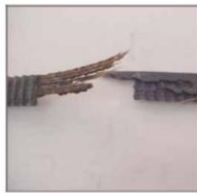
Figure 1. Normal fatigue failure [2]
