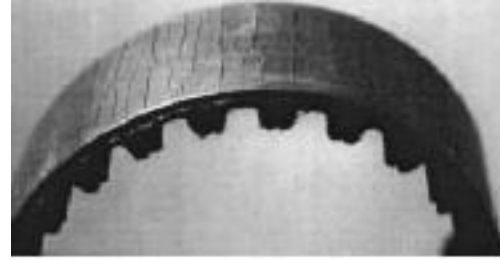
Figure 20. Back Cracking from high temperature[6]
