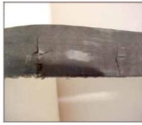
Figure 22. Tensile cord failure from debris [2]
