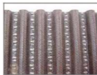
Figure 9. Excessive land area wear [2]
