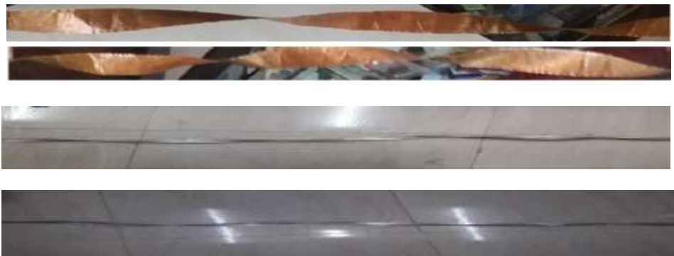
Figure: 2. Copper and Aluminium twisted tape ( y = 5.0 and 7.0 )
