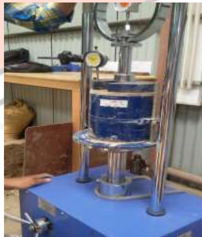
Fig 2. CBR test being conducted in the laboratory
