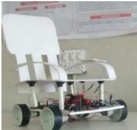
Fig: Exprimental model for touch-pad and voice command based wheelchair
