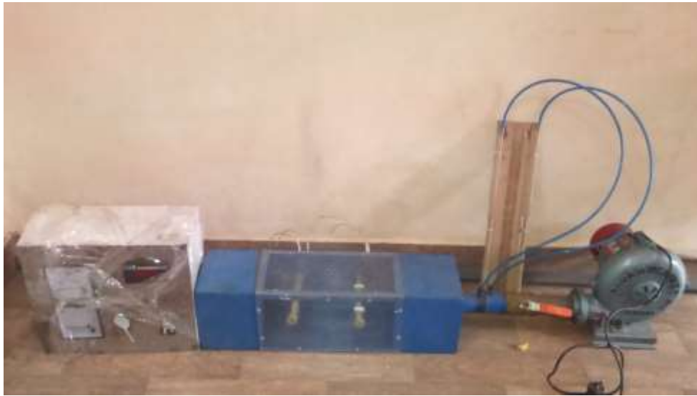
Fig 4.7 Duct system with acrylic
