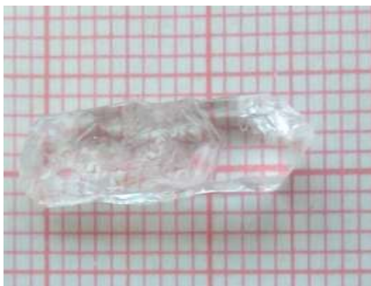
Figure1. As grown single crystal of LIADP
