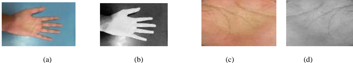
Figure 1. (a) Input image of Hand (b) Obtain Binary hand image from the Input (c) Extracted Palm print Image (d) Palm print Image in Gray scale Intensity Format
