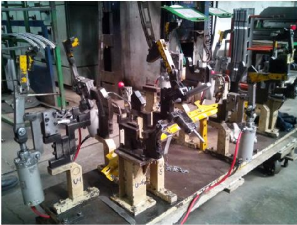
Fig.5 Pneumatic clamps mounted on welding fixture system
