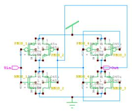
Figure 3.Schmitt Trigger Circuit design
