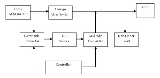
The DFIG draws a lagging volt-ampere reactive (VAR) for its excitation to build the rated air gap voltage. It is calculated from the machine parameters that the lagging VAR of 2.And when concerned to the USC rating the kVAR is needed when it is running as a motor. The operating speed of DFIG ranges from 0.7 p.u to 1.3 p.u. thus the maximum slip (s max) is 0.3. to make unity power factor at the
