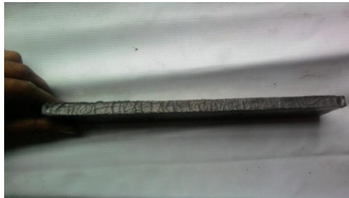
Figure 1 Paste coated mild steel plate
