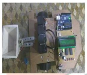
MODE 1: SEEDING, this mode adds seeds or fertilizers to the land, a vibrators is attached to the container, the vibrator is activated to the mode 2 command.
