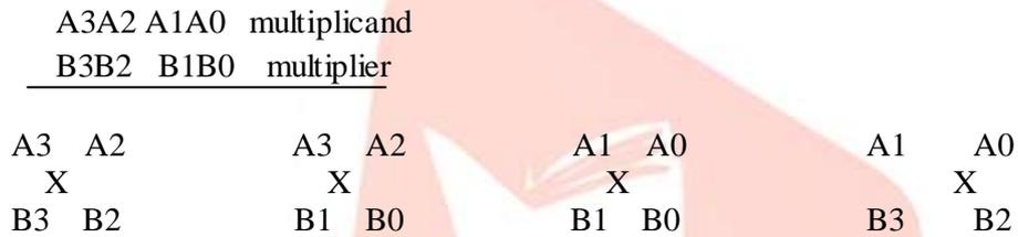
Figure 3: The Vedic Multiplication method for two 4-bit binary numbers
