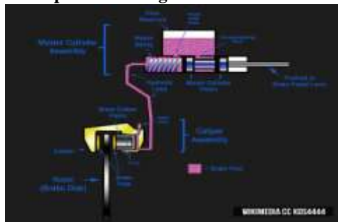
Fig.1 Principle of working of disc brake Fig.2 single-piston floating caliper disc brakes
