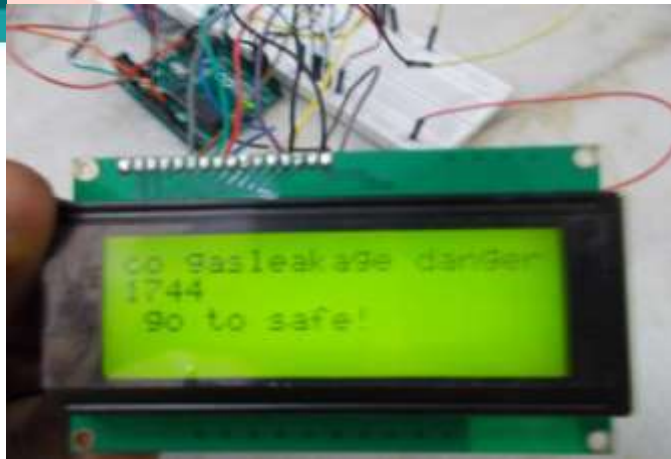
Figure7. Hard ware Output of co gases in LCD
