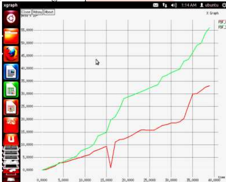
Fig9.Comparing Packet Drop Ratio
