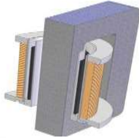
Figure.5: Inductive FCL concept with saturated iron core
