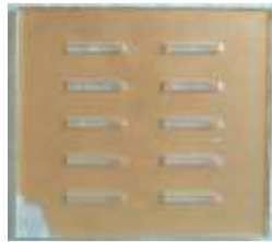
Figure. 2 Mould (acrylate sheet) for Impact test specimens
