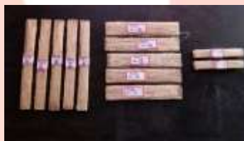
Figure.4 Specimens of Pine Apple Leaf Fiber – polyester resin for Tensile, Flexural and Impact tests
