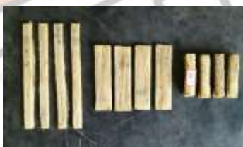
Figure.5 specimens of jute-pineapple leaf fiber-polyester resin Hybrid Composite for tensile, flexural and impact
