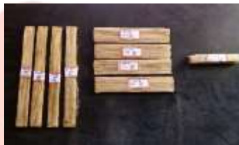
Figure.3 Specimens of jute – Polyester- resin for Tensile, Flexural and Impact tests
