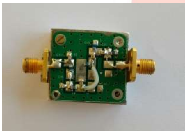
Figure 24. Fabricated filter of 50 to 100 MHz BPF
