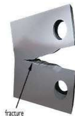
Figure: 5 Fracture CT specimen
