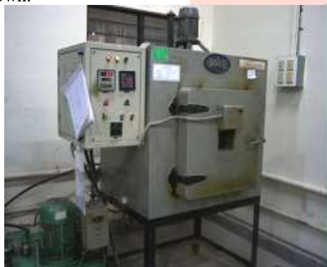
Fig 6: High temperature Oven and preparation of specimen as per ASTM standard using water jet cutting machine
