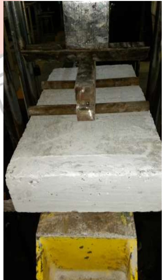
Figure 7: Two point load test setup
