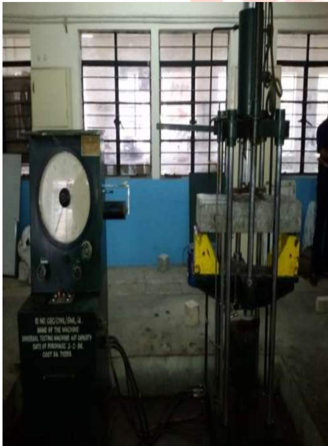
Figure 6: Universal Testing machine (40 ton capacity)
