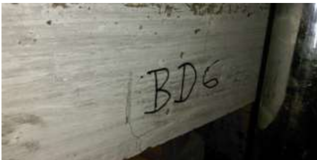
Figure 8: Flexure crack in specimen BD 6 of slab thickness 125 mm. Figure 9: Shear crack in specimen BD 8 of slab thickness 100 mm
