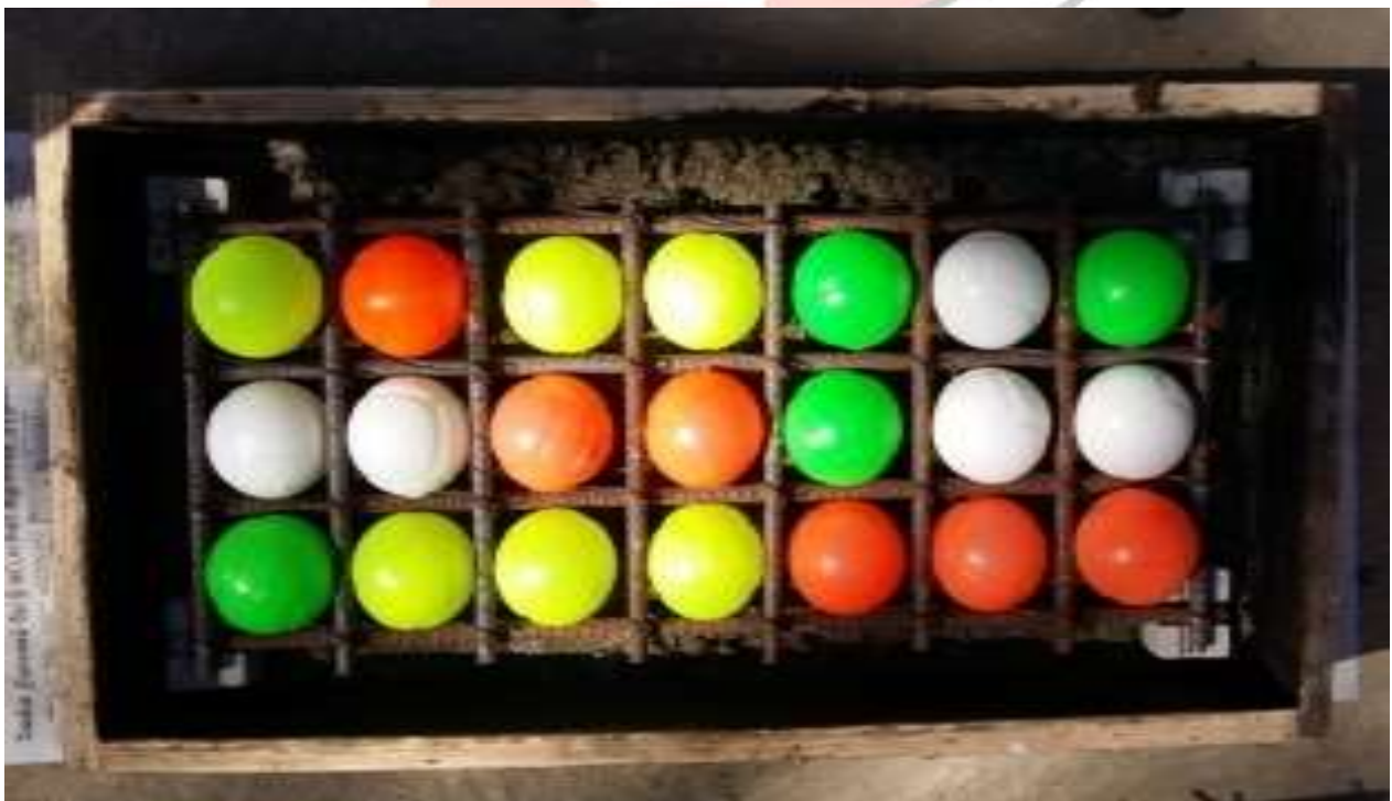
Figure 4: 60 mm diameter ball arranged at 20 mm spacing in a slab of size 600mm*300mm*100mm
