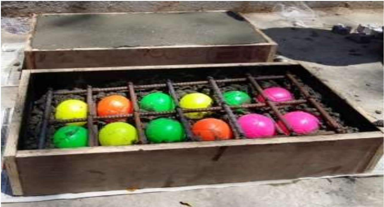
Figure 5: 75 mm diameter ball arranged at 20 mm spacing in a slab of size 600mm*300mm*100mm
