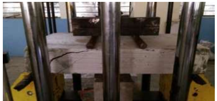
Figure 8: Flexure crack in specimen BD 6 of slab thickness 125 mm. Figure 9: Shear crack in specimen BD 8 of slab thickness 100 mm
