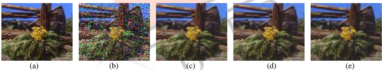
Figure 3. the image frames and their zoomed region are shown in the first and the second row. (a): original frame; (b) noisy frame with ( \sigma = 50, k = 5, s = 10\% ) (c): denoised frame by the VBM3D method; (d): denoised frame by the PCA-based method (d): denoised frame by our low-rank matrix completion algorithm.
