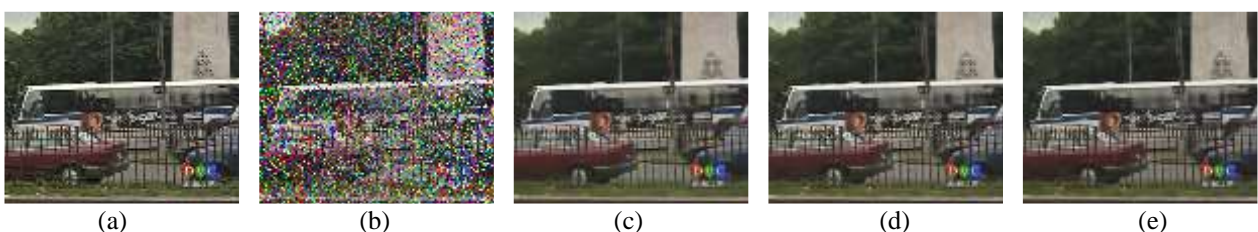
Figure 4. the image frames are shown. (a): original frame; (b) noisy frame ( \sigma = 20, k = 5, s = 30\% ) (c): denoised frame by the VBM3D method; (d): denoised frame by the PCA-based method; (d): denoised frame by our low-rank matrix completion algorithm.
