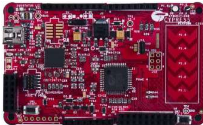
Fig4: PSoC 4 development board
