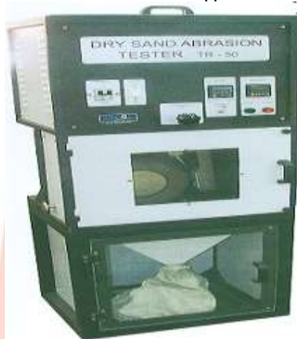
Fig 4: Dry sand tester
