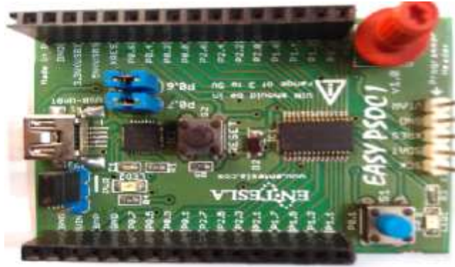
Figure 2 Development Board of PSOC1 (CY8C28433)
