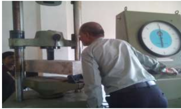
Figure 3. Flexural test setup
