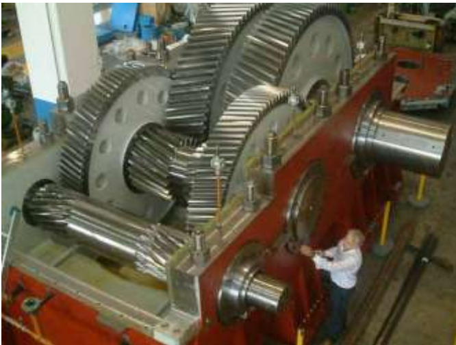
Fig.5 Double helical gear of a cement mill rotary gear drive
