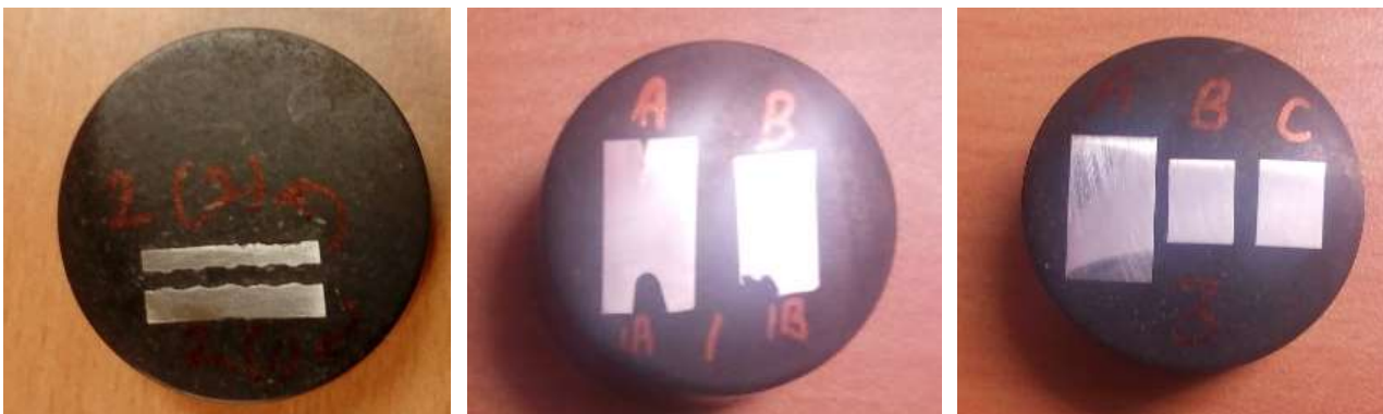
Fig. 1: Turbine blade specimens mounted in Bakelite
