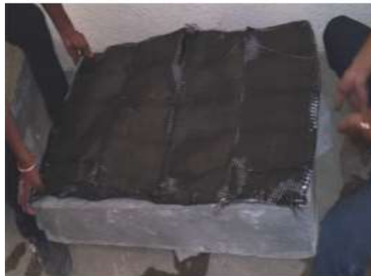
Fig. 8: Slab Panel using CFRP/GFRP Sheet
