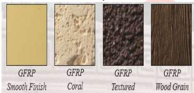
Fig. 2: Different Texture of GFRP sheet
