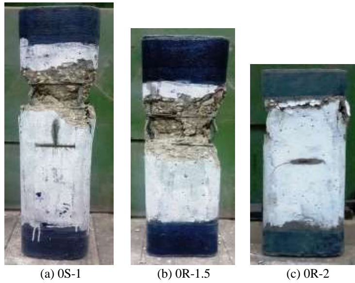
Figure 5. Failure mechanism (FM1) for unconfined RC columns
