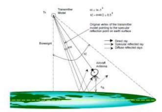
Fig.5 Satellite to aircraft ray tracing model
