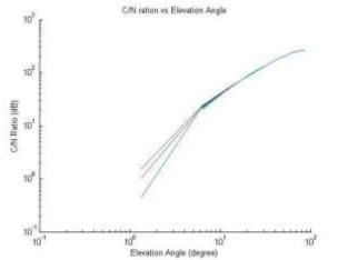
Fig.6(k): ):c/n ratio vs elevation angle with rms height 5m **REFERECES**
