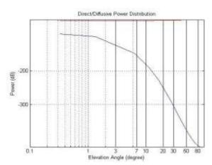
Fig 6(d): Direct/Diffuse Signal Power Distribution
