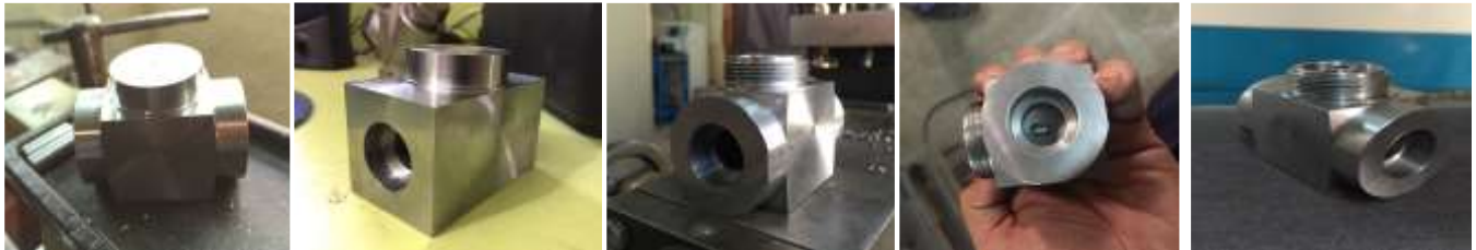
Fig 2-Shows the development stages of manufacturing of steam trap
