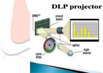
Fig. 6. Digital Light Processing Projector
