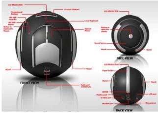
Fig. 2. Element of E-ball computer
