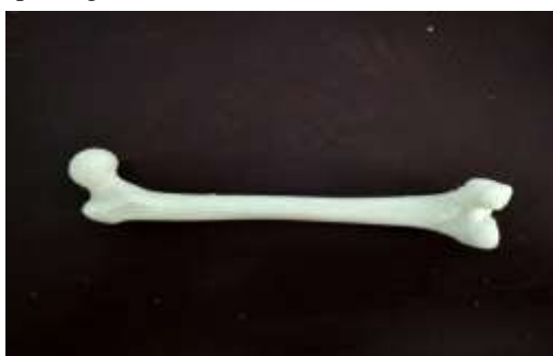
Fig 5.4: Our final 3D Printed Femur Bone
