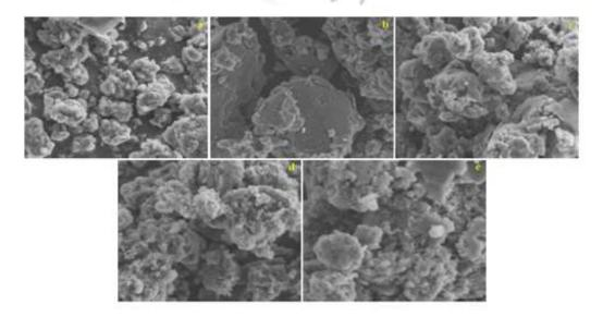
Figure 1: SEM micrographs of PANI/NiO composites with different NiO content: (a) 10, (b) 20, (c) 30, (d) 40 and (e) 50 wt%.
