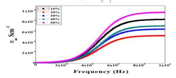
Figure 3: AC conductivity of PANI/NiO composites as a function of frequency for different NiO content.
